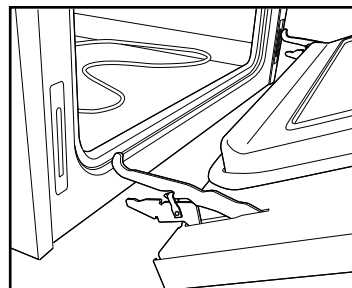
Door removed from the range.
